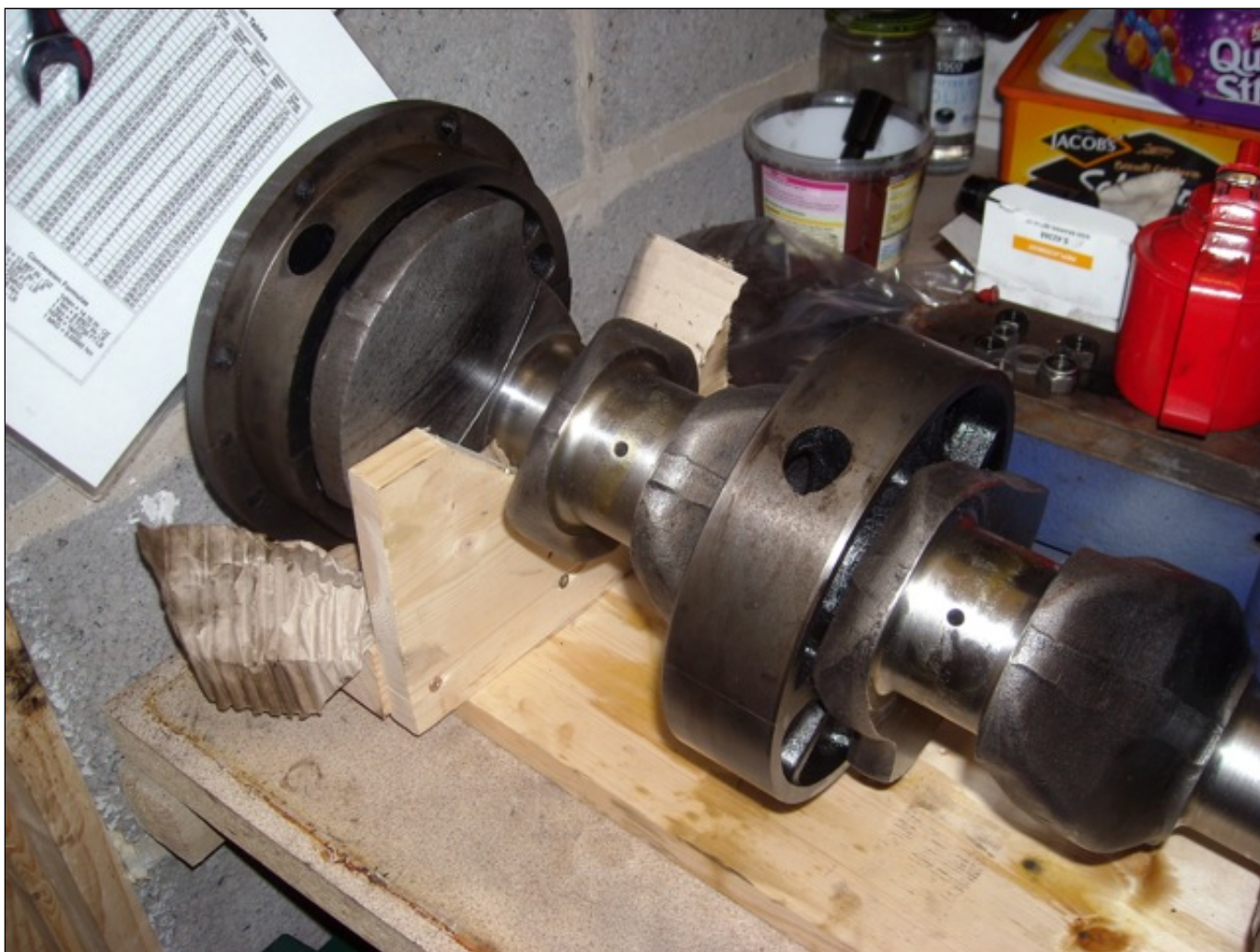
The back and centre bearing housings assembled. the front is fitted once the shaft is in place.
